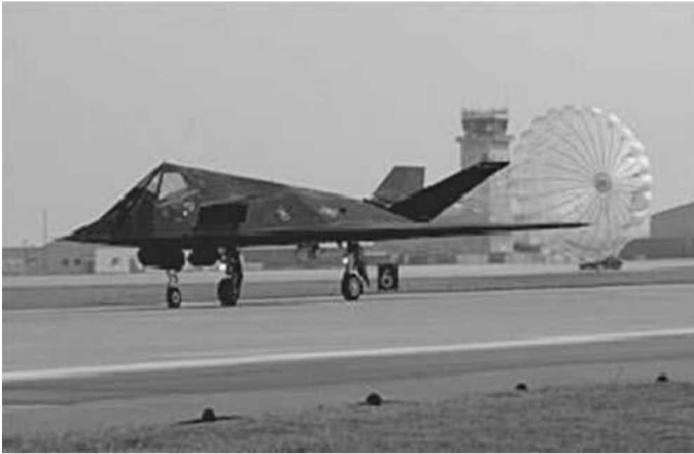
Figure F117 deploying brake parachute (Courtesy of US Air Force/ Senior Airman Darnell Cannady)
