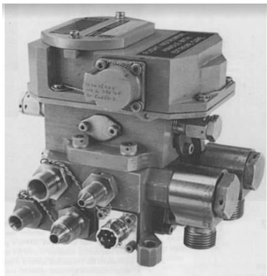
Figure 2.11 is a photograph of a 'Q' feel unit supplied by Dowty for the BAE Harrier GR5 and McDonnell Douglas AV-8B aircraft.
